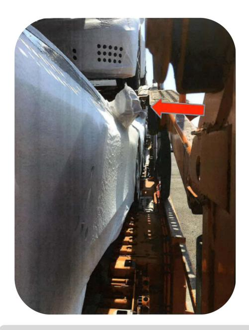
A-1 position (#7) if backed in must be center on the deck or the mirrors will be hit by B-2 deck (#2).
