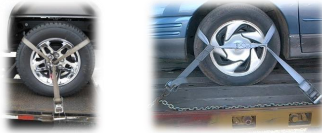
Figures 4 and 5: One point and two point soft-ties – NOT permit
