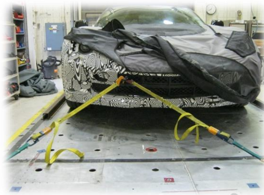
Figure 6: Front eye bolt on right side of fascia through the grille.
