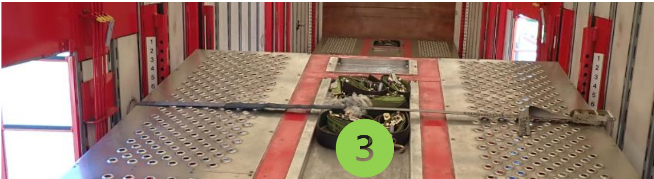
Figure 6 *image is of the front of table 3 in the up position and ratchet applied to stabilize.
